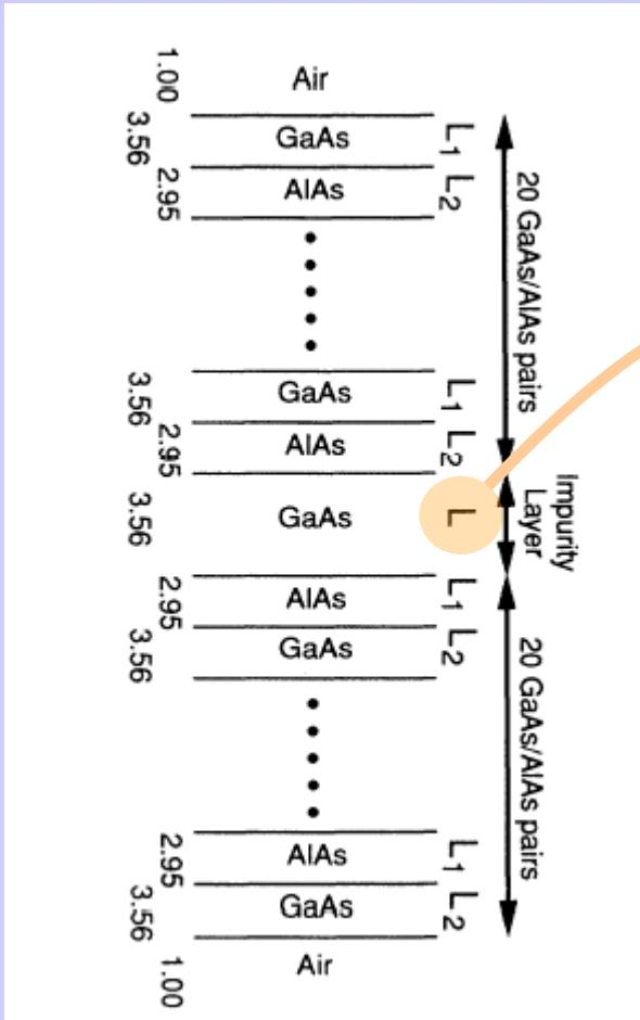
⇒ varying the height of one layer introduces an **impurity state** in the gap
