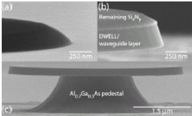
FIG. 1. Scanning electron microscope images of DWELL-containing micro-disk cavities after the (a) Si<sub>3</sub>N<sub>4</sub> etch, and (b) and (c) AlGaAs etch and undercut.
