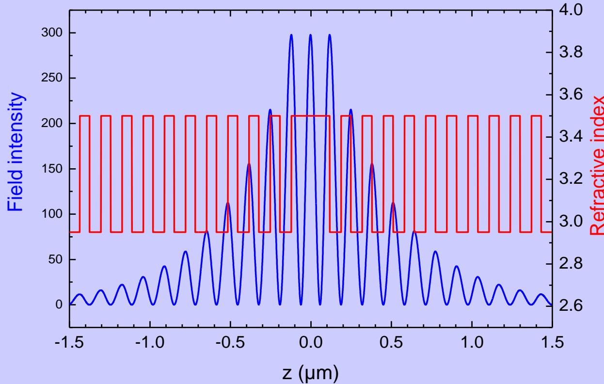
⇒ Field peaked at cavity center, exponential decay in the DBRs
