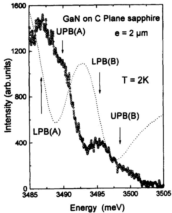
Fig. 1. 2 K reflectance spectrum (dashed line) and the corresponding 2 K photoluminescence (open circles) spectrum which shows the LPB and UPB contributions to the GaN fluorescence.
