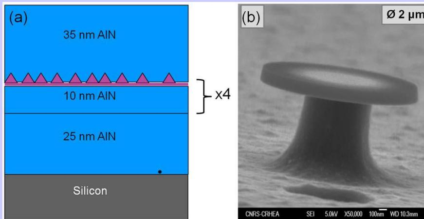
GaN quantum dots in AlN slab on Si
