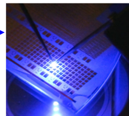
In 0.2 Ga 0.8 N-based blue LEDs emitting near 450 nm
